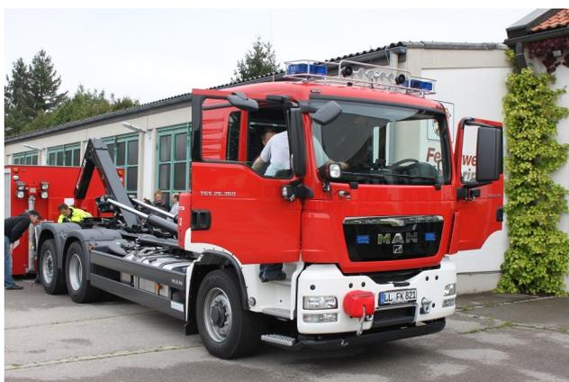
Haken: 20t Hubkraft, 14t maximale Container-Masse
